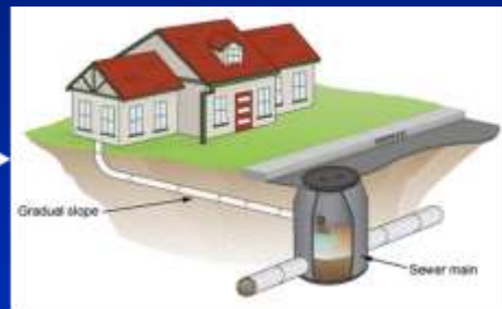
Conventional Gravity Sewer
